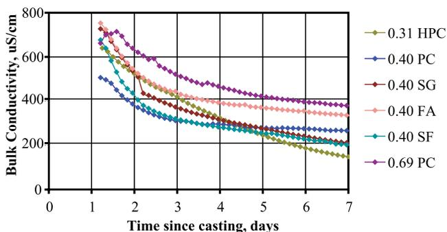
**Fig. 2: Bulk conductivity (at 3-hour intervals) versus time after casting to 7 days**
