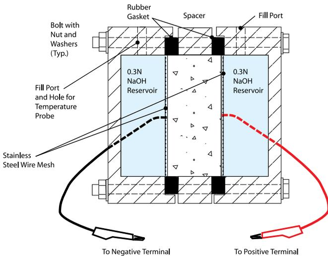
**Fig. 1: Schematic of conductivity testing apparatus**
