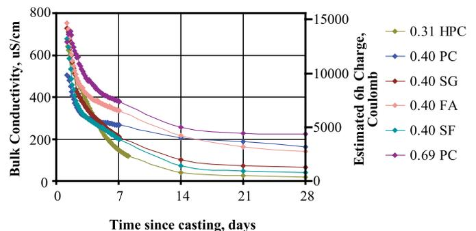
**Fig. 3: Bulk conductivity versus time after casting to 28 days**
