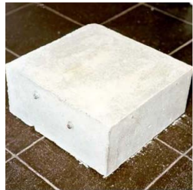
Figure 4: Specimen with rebars in different depths
