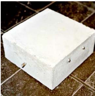
Figure 3: Specimen with parallel rebars and crossing
