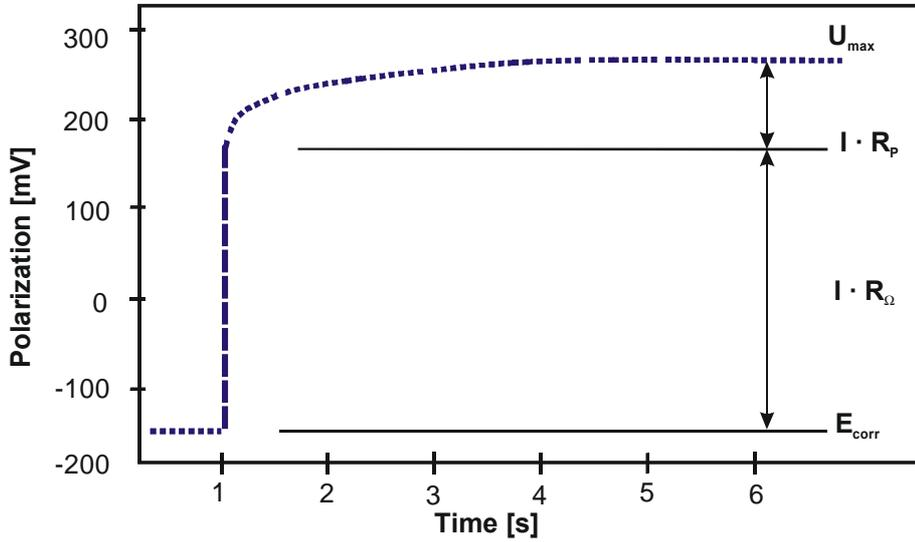
Fig. 1. Typical polarisation pattern
