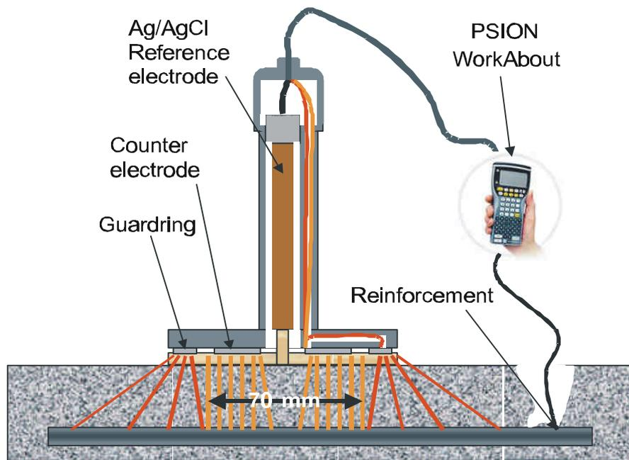
Fig. 2. Schematic setup showing the confined area.
