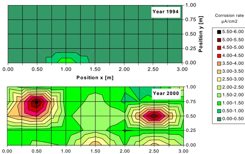
Fig. 4. 2D surface plot of corrosion rates measured by the galvanostatic pulse method in 1994 and 2000, respectively.
