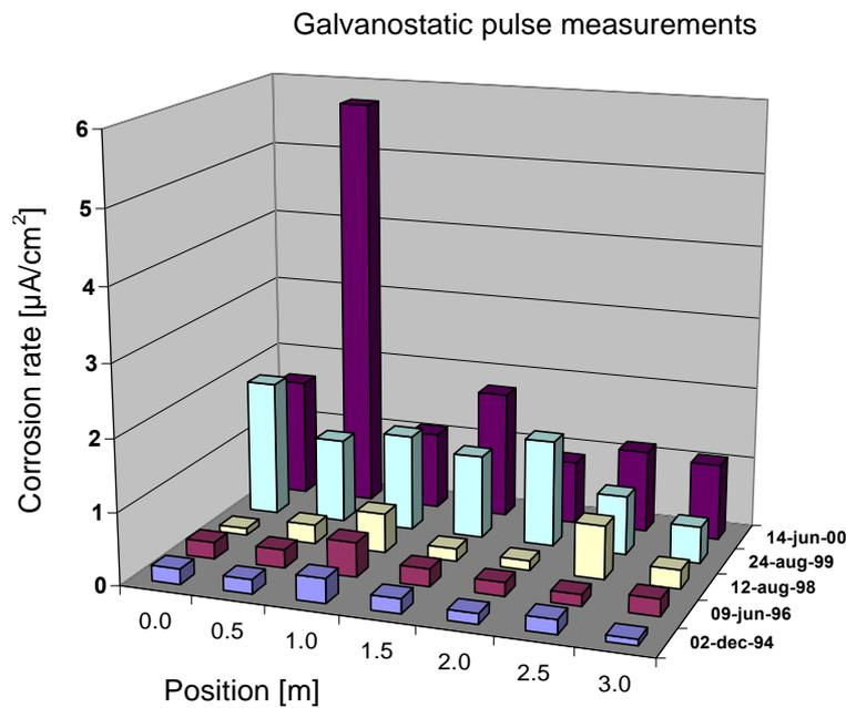
Fig. 3. Corrosion rates for reinforcement in bridge column at the height of 75 cm above ground. The measurements are done by GPM in the period 1994 - 2000.
