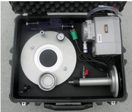
**B-10000 DSV-Kit:** For surface planing, bonding the disc, and attaching the coring rig to produce the partial core without anchoring.
