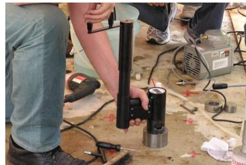
The procedure and special equipment used for the **BOND-TEST** ensure that the disc is loaded in direct tension without bending. Bending may lower results by 20 to 50 %. The discs have sufficient stiffness to avoid distortion during testing. By bonding a clean disc on a planed, dry surface with the GRA adhesive, failure should not occur at the disc/overlay interface. Failure at the disc/overlay interface is an inconclusive test and must be repeated if the bond strength is to be evaluated.
