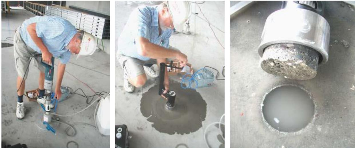
**BOND-TEST** being performed for quality control of the bond between a wear resistant overlay and a concrete slab; coring after bonding the 75- mm disc is shown (left), application of pull-off load (middle), and the bond failure, type (b), between the overlay and the substrate (right) at 1.8 MPa
