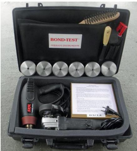
**B-11000 BOND-TEST Preparation Kit:** For removing the center knob after surface planing, cleaning the surface, bonding the discs, and heating the discs in cold weather conditions
