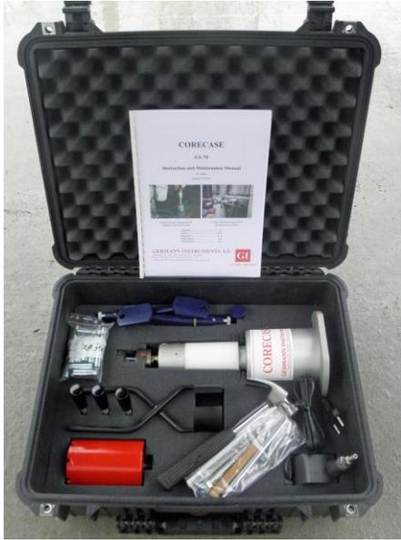
**CORECASE CS-75:** Coring device for producing the partial core.
