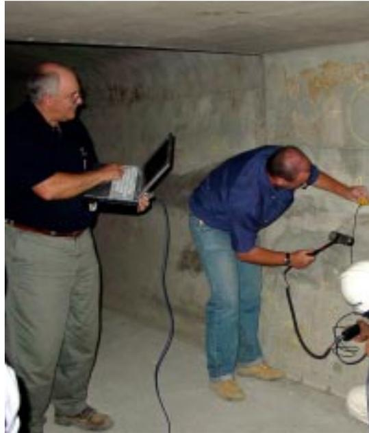
Fig. 7 Impulse Response Equipment.
