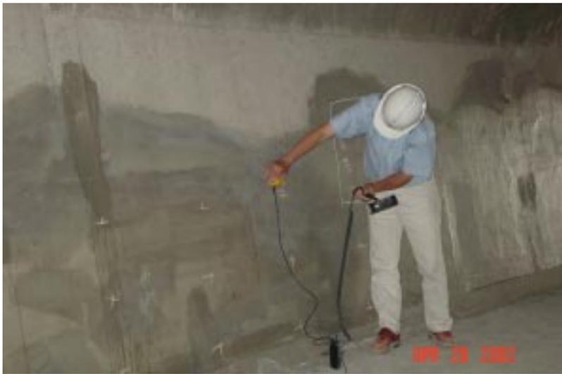
Fig. 9 IR Test on Girder Web.
