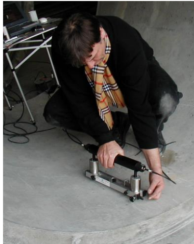
Measurement of P-wave speed by surface method
