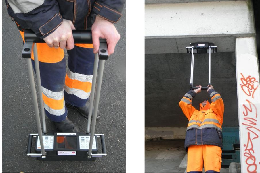
*Fig. 1. The extension handle mounted the MIRA antenna*
