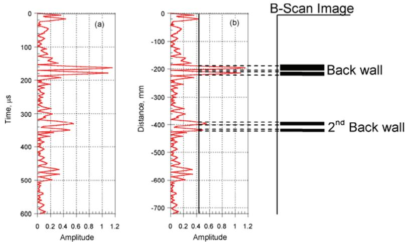
After the scanning is completed, the results can be displayed in two ways. The individual A-Scans can be analyzed or cross sections (B-Scans) along each scan line can be viewed. The following explains the approach used to construct a cross-sectional view of the test object and show the depth of reflecting interfaces. The signal at each test point is plotted with time in the vertical direction as shown in left hand figure (a). If the shear-wave speed in the concrete is known, the time axis
