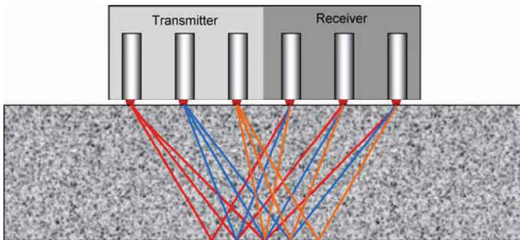
The averaged signal recorded by the receiving transducers is stored in the hand-held unit as a time-domain waveform. An example of such a waveform is shown at the top of the next page. In this case, the test was done on a solid concrete slab with a thickness of about 200 mm. The figure on the left side of the next page shows signal amplitude as a function of time (**A-Scan**). The three peaks are due to multiple reflections
