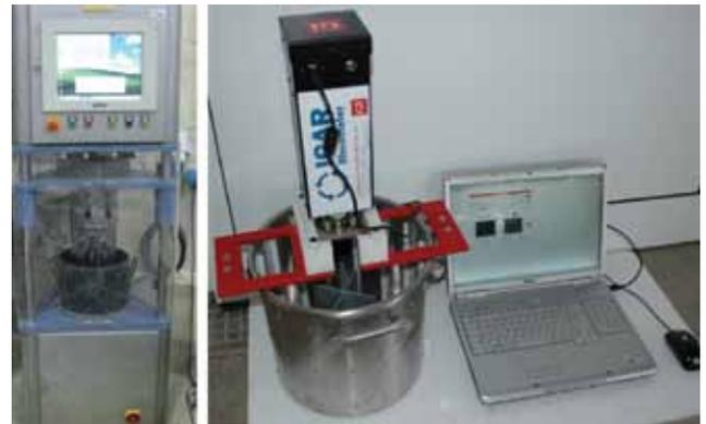
Figure 2. Rheometers, ConTec Viscometer 5 (left), ICAR Rheometer (right)
