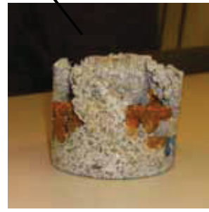
Core with voids below bars
