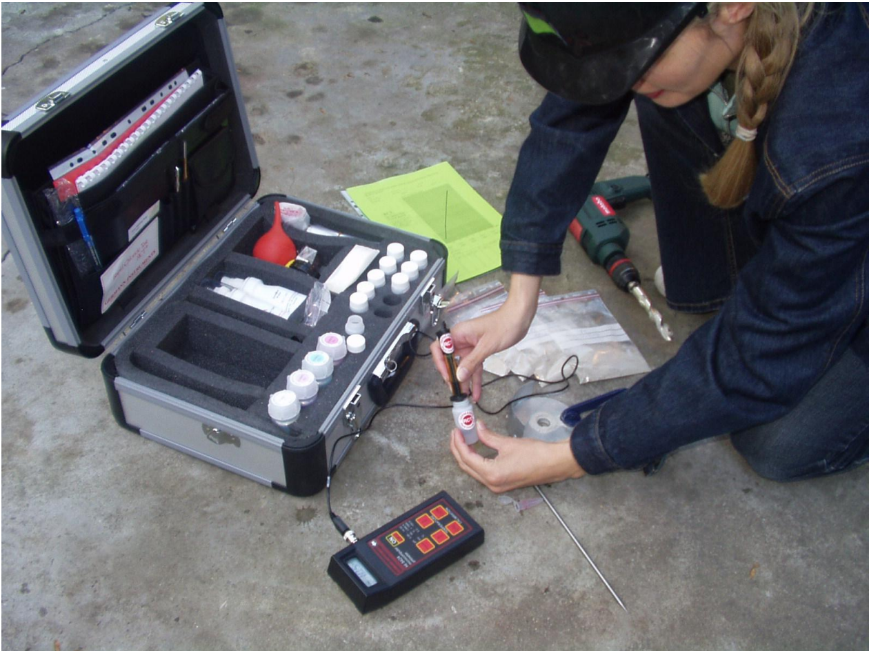
RCT measurement performed on-site
