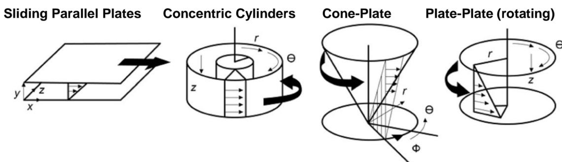
Fig. 1: Four examples of how to deform a material between two surfaces
