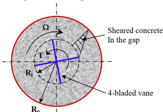
Fig. 3: Principle of a rheological test using ICAR Plus
