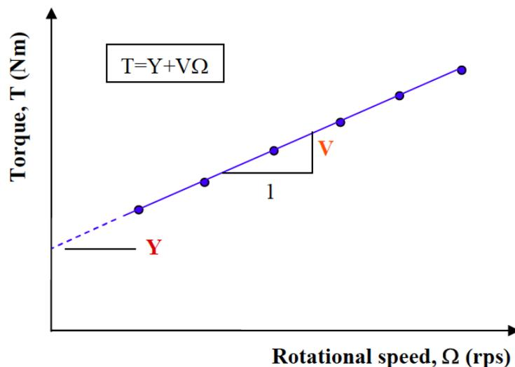
Fig. 6: How the Y-value and V-value parameters are obtained in a flow curve test
