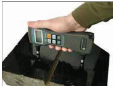
Measure transit time ( t_c ) across crack
