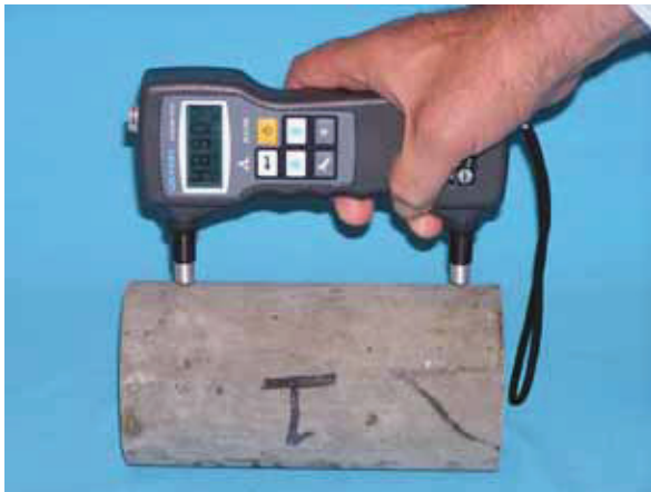
Measure transit time ( t_p ) parallel to crack
