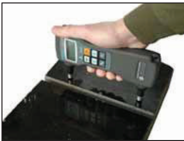
Measure transit time ( t_p ) parallel to crack
