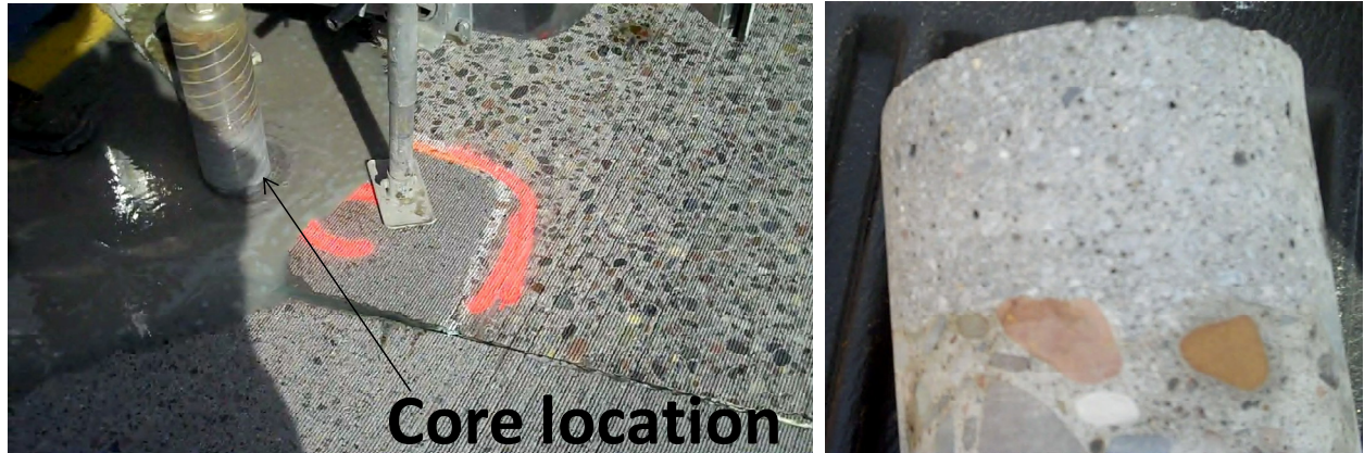
Figure 7. Core location (left) and result showing properly bonded partial depth repair.
