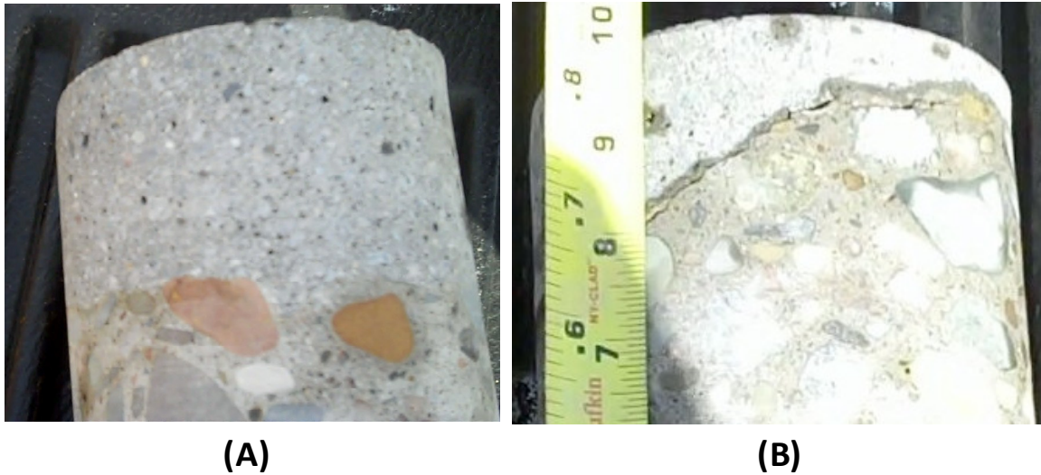
Figure 10. Cores taken at the area (B) towards the centerline near the transverse joint indicating an improperly bonded partial depth repair in comparison to (A) the properly bonded repair.
