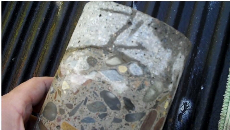
Figure 11. Core showing debonding of the partial depth repair.
