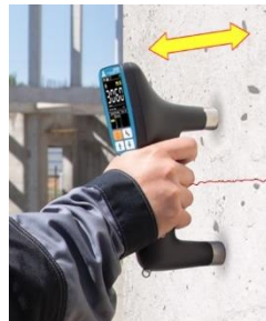
Measure transit time ( t_c ) across crack
