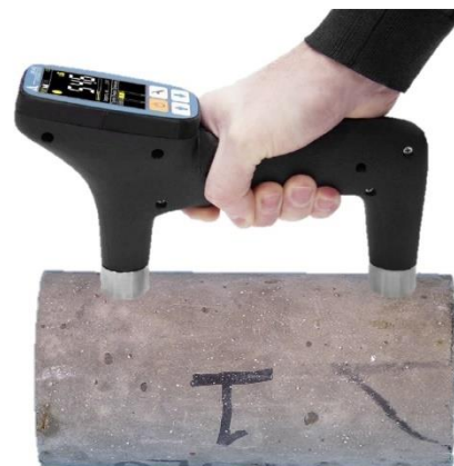
Display of transit times and crack depth
