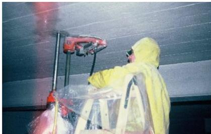
Broke the core and drilled a center hole, 8 mm in diameter, planed the surfaces for a 25 mm distance, inserted a LOK-TEST disc from below and threaded it into a pull bolt from above, connected to the LOK-TEST pull machine. Tested to failure and got 28 kN as the pull force. One test lasted 1 day.
