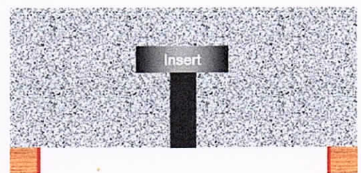
Figure 2. The formwork (or part of the formwork) and the stem of the test bolt are removed.
