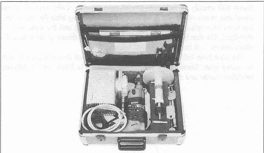
Figure 19. CAPO-test suction plate with diamond surface planing wheel.
