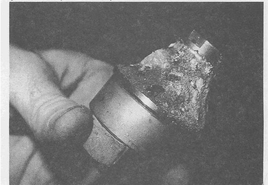
Figure 59. Detail of the CAPO-test pull-out cone.
