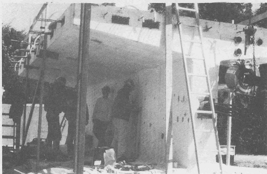
Figure 35. At the final examination of the technicians performing the pull-out testing. Each technician has to test 6 LOK-test inserts, 6 CAPO-test inserts on-site, report the results and check the test equipment to be in workable condition.
