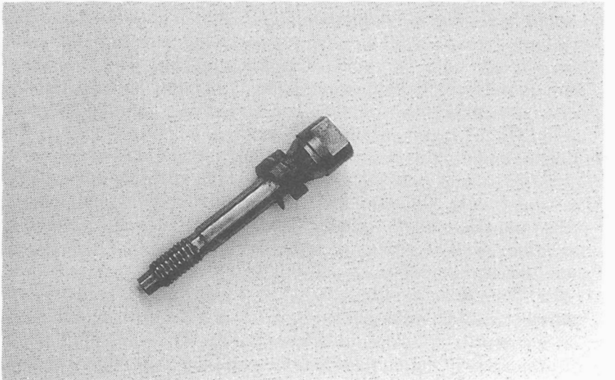
Figure 23. The CAPO-test insert is put on the cone pullbolt with the inner sharp edge facing the cone.
