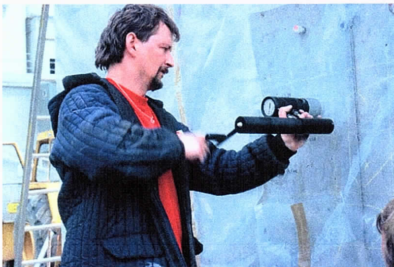
Fig.16. LOK/CAPO-Test in progress.
