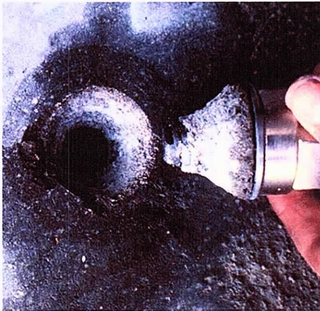
Fig. 4—Example of unacceptable CAPO-TEST; surface was not flat and a complete ring was not formed at surface.
