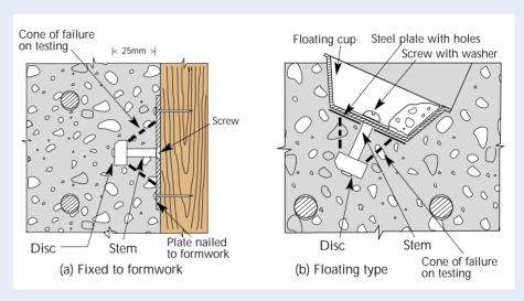
Figure 3: Lok-test inserts.
