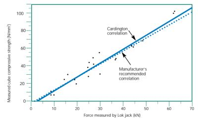
Figure 5: Correlation of Lok-tests and cube tests carried out at Cardington.
