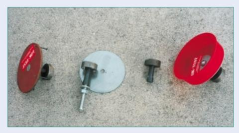
Figure 4: Lok-test inserts for formwork (left) and floating cup (right)
