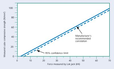
**Figure 2:** Illustrative correlation between strengths determined by the Lok-test and by conventional cube testing.
