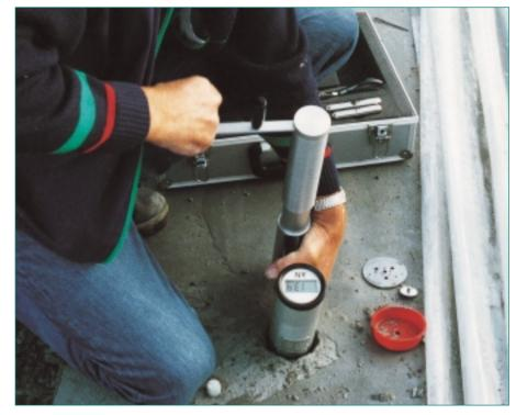
Figure 1: the Lok-test jack in position.
