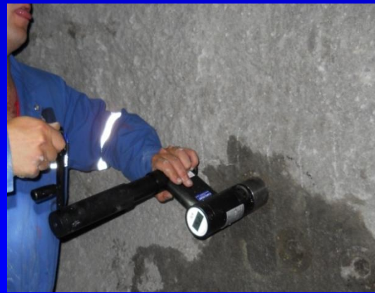
Cigar Lake Uranium Mine, CA Strength of granite concrete Test smart – Build right
