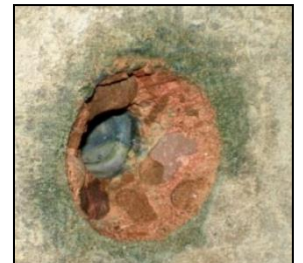
Rainbow Indicator sprayed on the CAPO-TEST cone hole, pH < 5 (red color)- totally carbonated
