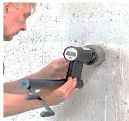
Mounting the hydraulic pull machine, ready for pull-off
