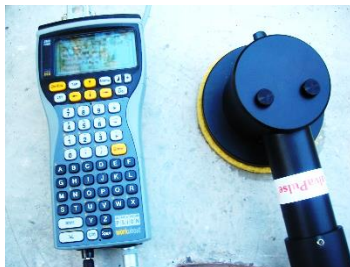
GalvaPulse for corrosion rate, half-cell potentials and electrical resistance of the cover layer, corrosion rate 3D-mapping shown
