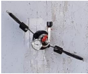
GWT, Germann's Waterpermeation Test. A selected water pressure is maintained by the micrometer gauge pressing a pin into the water chamber measuring the amount of water penetrating the concrete
