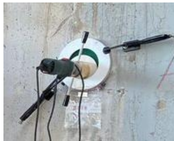
Profile Grinding, followed by testing for chlorides on-site with the RCT of the concrete powders and establishment of a chloride profile for service life estimation
