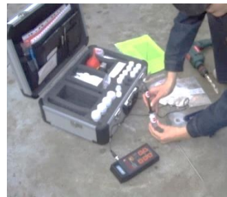
Profile Grinding, followed by testing for chlorides on-site with the RCT of the concrete powders and establishment of a chloride profile for service life estimation
