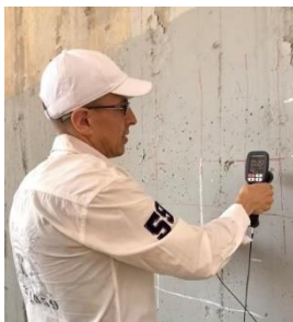
Surfer for surface wave speed and depth of surface opening cracks < 100 mm
