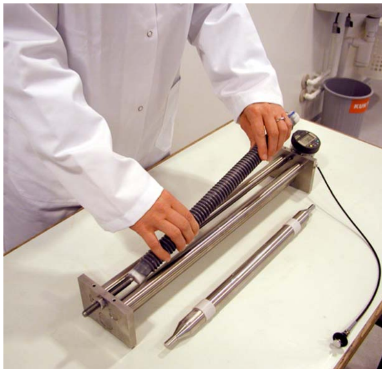
NOTE—Notice the mark with permanent ink at one end of the specimen showing the upside and measuring gauge position during measurements. FIG. 9 Placement of Specimen in the Dilatometer Bench for Length Measurement
