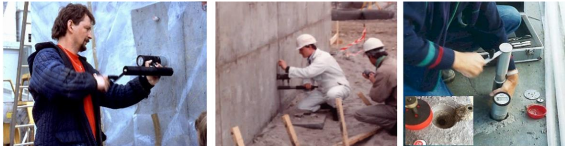
Figure 38. Left: Great Belt Link, Denmark, 40,000 pullouts were made. The strength by pullout was accepted if the strength was minimum 80% of the potential lab strength [16]. Center: supporting sea wall, Copenhagen. Minimal curing compound applied. Pullout strength = 70% of lab strength. Right: Garage parking structure, UK. Concrete covered by heavy plastic sheet and wet mats. Pullout matched the lab strength.
