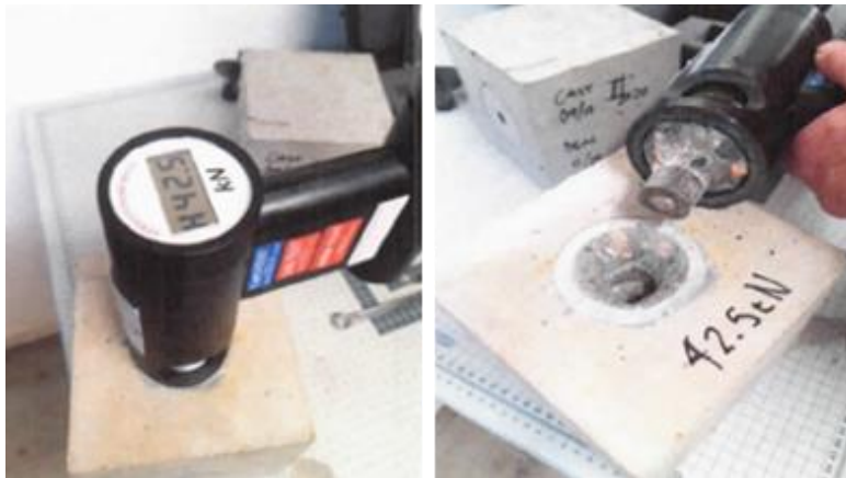
Figure 35. LOK-TEST pullout force in kN, testing depth 25 mm.
