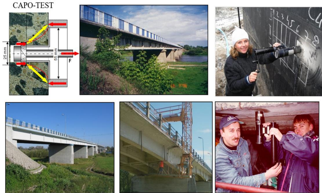
Figure 39. Examples of Polish bridges tested for upgrading –higher loading– shown with CAPO-TEST
