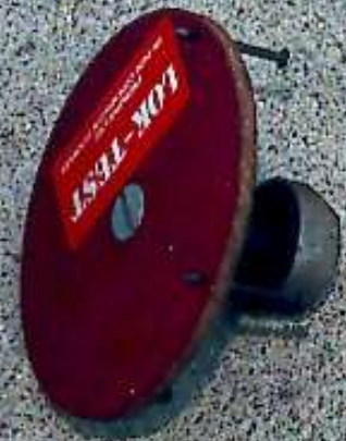
Nailed to formwork
