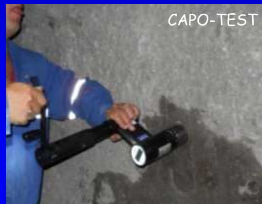
Cigar Lake Uranium Mine, Canada Strength of gunite concrete Test smart – Build right
