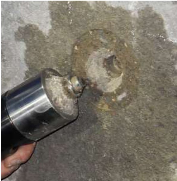
The completed CAPO-TEST. Notice the unfolded CAPO ring on the cone pull bolt.
