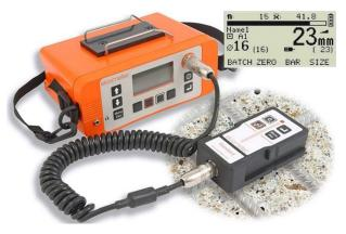
pitch and the signal strength indicator bar on the display increases in length. When the bar is positioned below the center of the search head, the pitch of the sound will be at its highest and the signal strength indicator bar will be at its maximum. At this moment, the depth of cover will be shown on the display.
