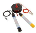
Suitable for models BH, SH, TH and THD. Consists of either a copper / copper sulphate electrode or a silver / silver chloride electrode. Each half cell is a sealed unit, no need to mix chemicals.
