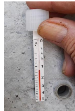
COMA-Meter integrating temperature and time, here showing 1.2 M 20 days (days at 20°C)
