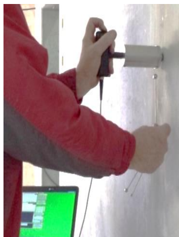
Joint tested for voids
