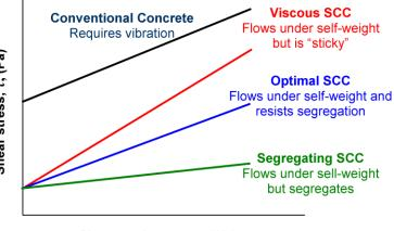
Shear strain rate,  $\dot{\gamma}$ , (1/s)
