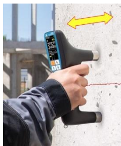
Measure transit time ( t_c ) across crack
