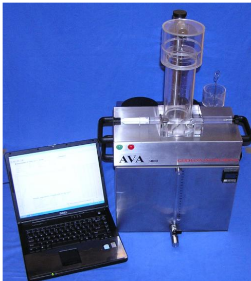
AVA-3000 System consisting of laptop with installed software, base unit, riser column, water tank and sampling equipment.
