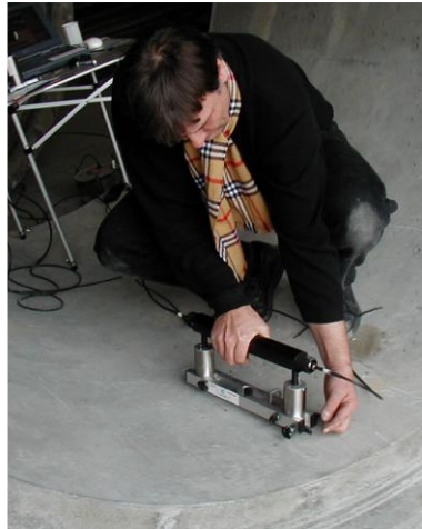
Measurement of P-wave speed by surface method
