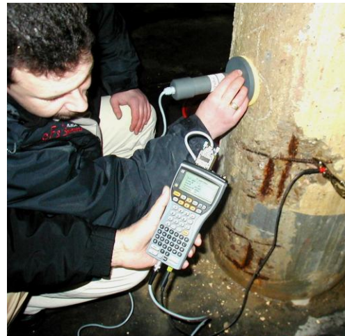
GalvaPulse (older model) testing in progress for corrosion activity of a heavily corroded column
