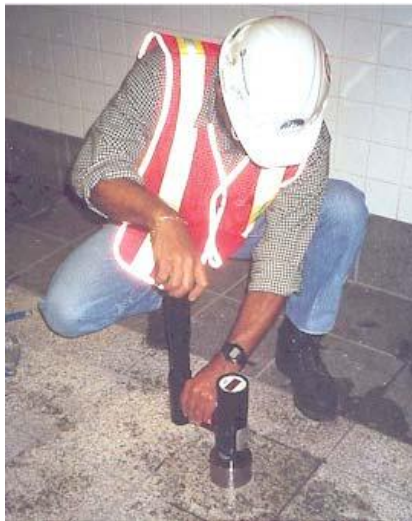
BOND-TEST being performed on granite tiles in a subway station
