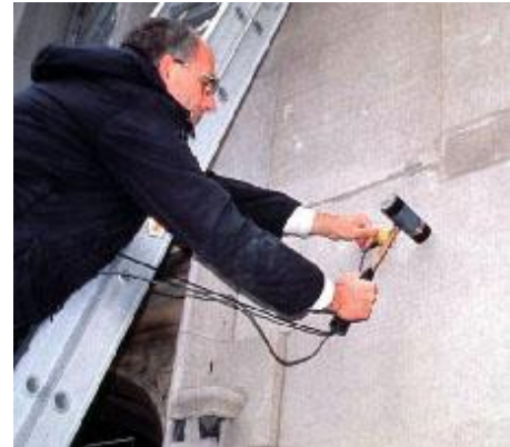
Dr. Allan Davis testing the stiffness of concrete segments in Wrigley Building, Chicago, USA
