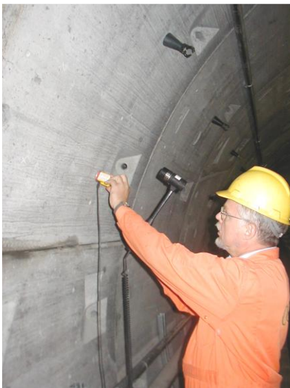
Testing for voids behind tunnel lining
