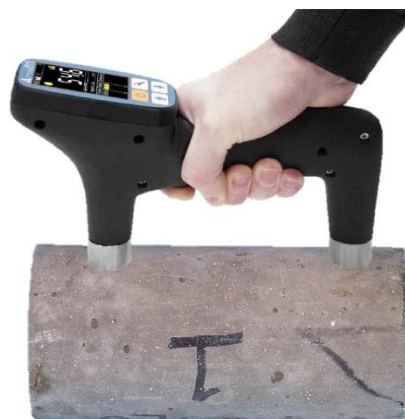
Display of transit times and crack depth
