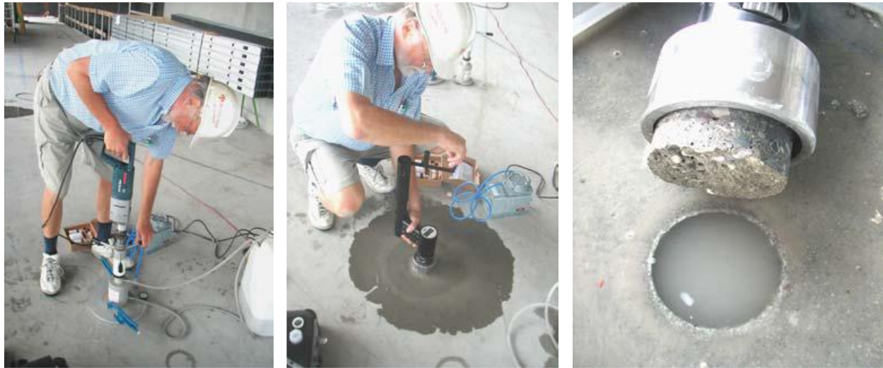
BOND-TEST being performed for quality control of the bond between a wear resistant overlay and a concrete slab; coring after bonding the 75- mm disc is shown (left), application of pull-off load (middle), and the bond failure, type (b), between the overlay and the substrate (right) at 1.8 MPa
