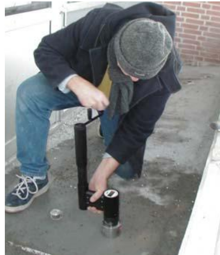
The bond of a repair on a balcony being evaluated with BOND-TEST
