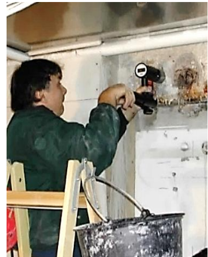
Dubious beam being tested for strength, Denmark
