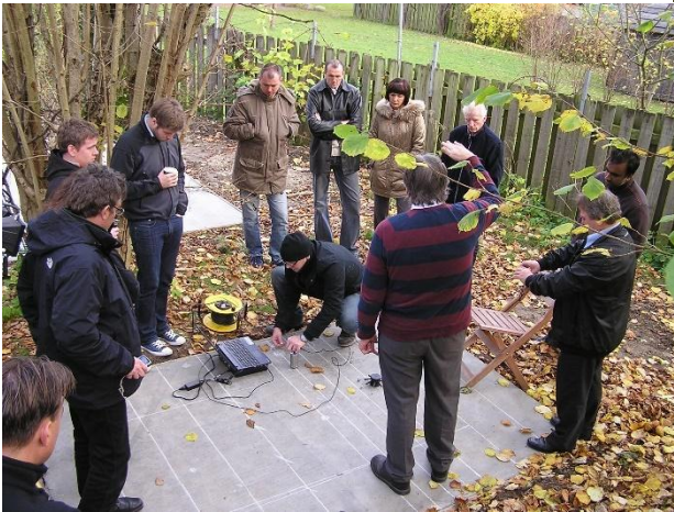
Outdoor facility in Copenhagen includes two 400 mm thick slabs with various simulated defects
