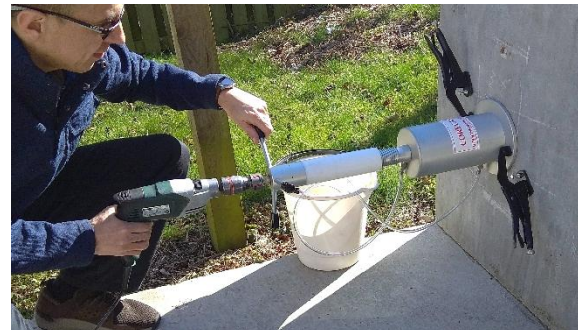
Coring with the CEL-100 rig to for testing chloride permeability over the specimen
