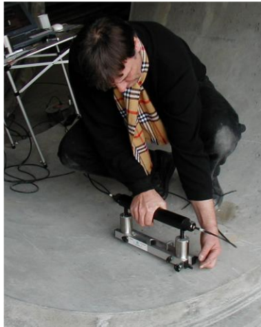
Measurement of P-wave speed by surface method
