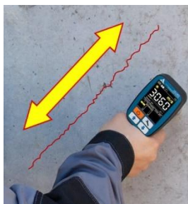
Measure transit time ( t_p ) parallel to crack
