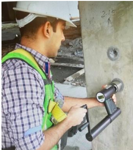
Column being tested for strength acceptance, Mexico
