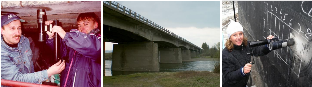
Strength evaluation of 15 bridges (25 to 52 years old) on carbonated concrete, Poland
