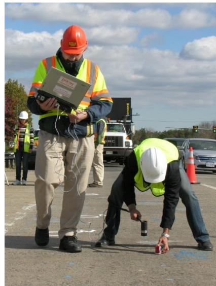
Testing for delaminations in bridge deck
